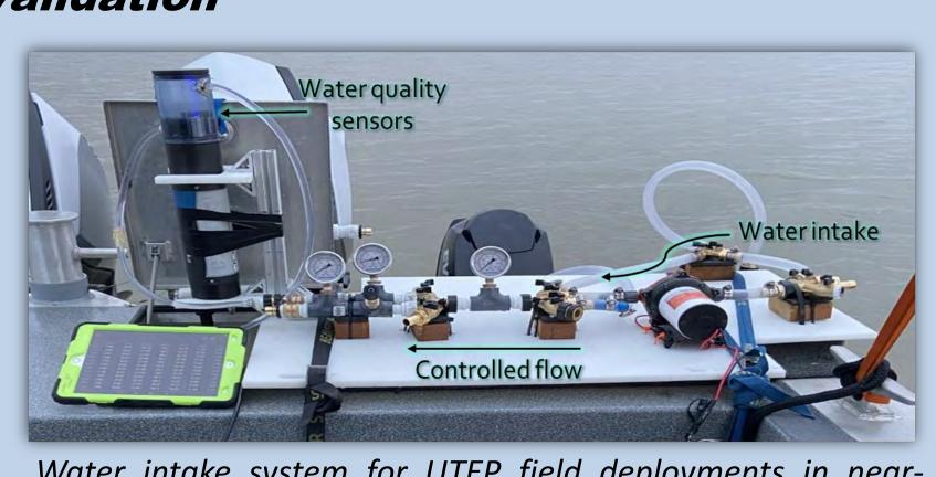
Water intake system for UTEP field deployments in nearshore aquatic environments, developed summer 2022 This system as used while the research vessel was moving.
