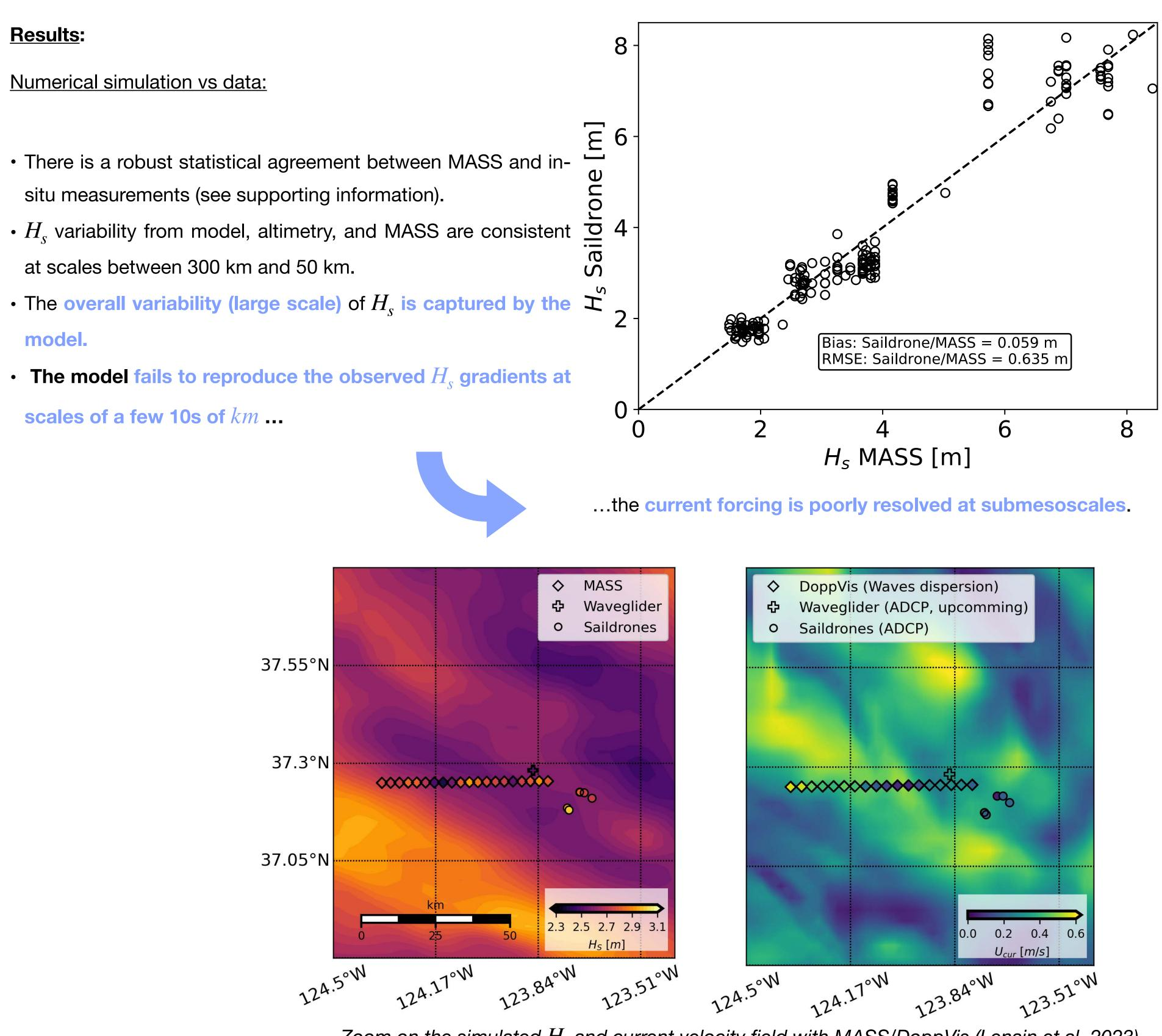
Zoom on the simulated  $H_s$  and current velocity field with MASS/DoppVis (Lenain et al. 2023) and autonomous platform measurements
