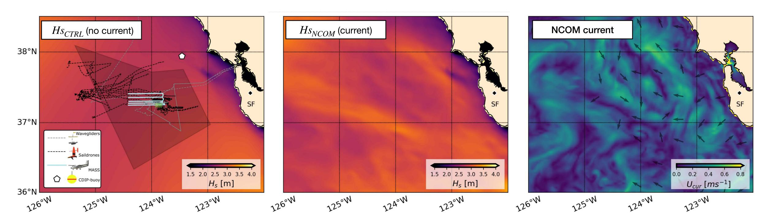
Snapshot of simulated  $H_s$  (WAVEWATCH 3) without (CTRL) and with (NCOM) current forcing during the S-MODE Pilot campaign.
