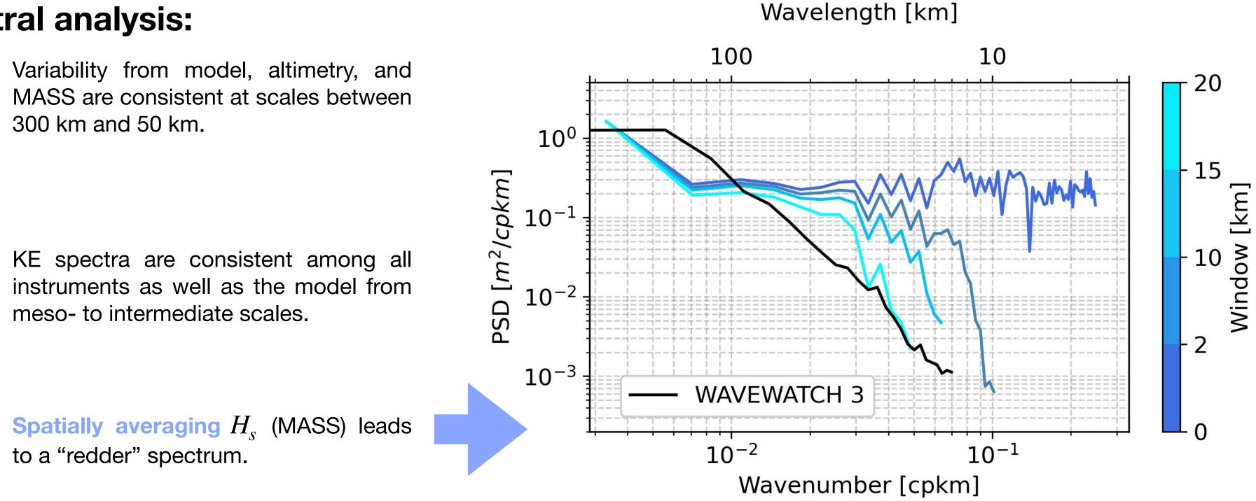
Averaged wavenumber spectra of  $H_s$  measured by MASS and model.  $H_{\rm s}$  measured by MASS have been smoothed at different scales with a moving average
