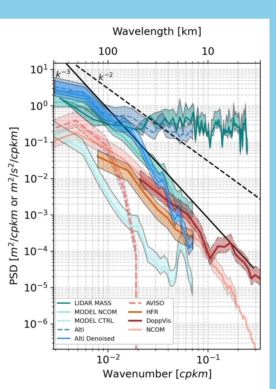
Wavenumber spectrum of: significant wave height (blueshade) from model, altimetry, and MASS data energy from model, HFR, AVISO product, and DoppVis *instrument (red-shade)*
