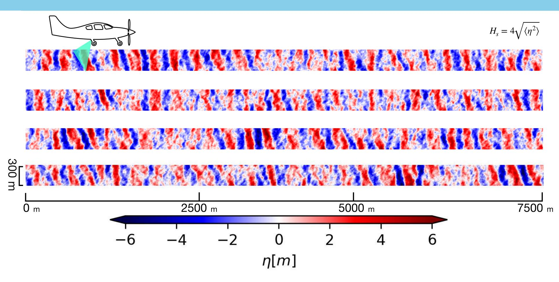
Four 7500 m x 300 m swaths of sea surface height measured by the MASS instrument
