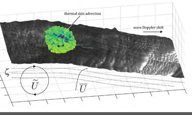
Stylized breakdown of the mean and wave orbital flow components  $\bar{U}$  and  $\tilde{U}$  underneath an undulating surface (in this case, the water surface displacement field produced through integration of the water surface slope field, supplemented with representation of skin brightness temperature). The fixed and interface following vertical coordinates z and  $\zeta$ are shown for reference.
