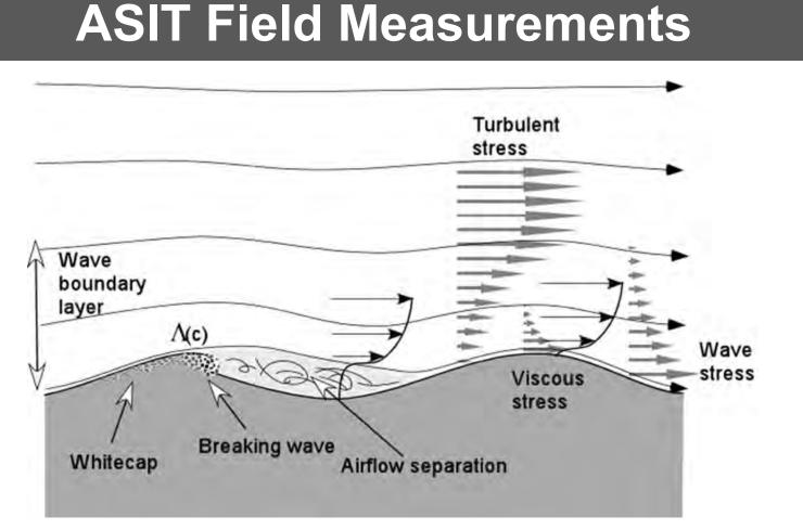
Conceptual schematic of the constant stress layer above the wave surface where surface waves break, create whitecaps, and induce flow separation. At the surface, the total turbulent stress is partitioned to the surface tangential viscous stress and
