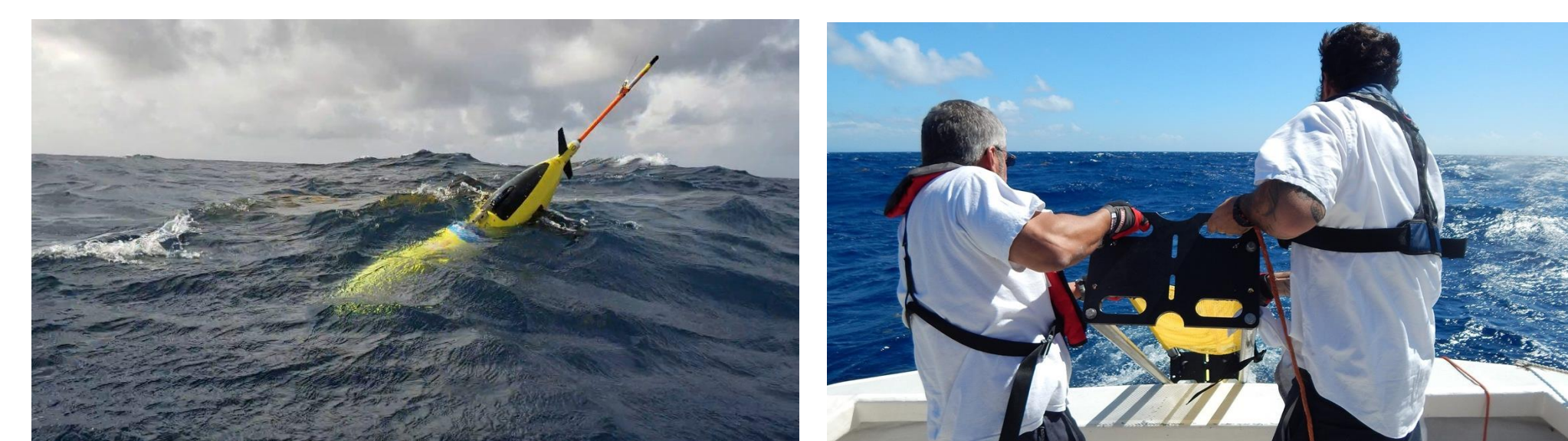
Figure 3. Underwater gliders propel themselves by using small buoyancy changes and wings to convert vertical motion into horizontal motion.
