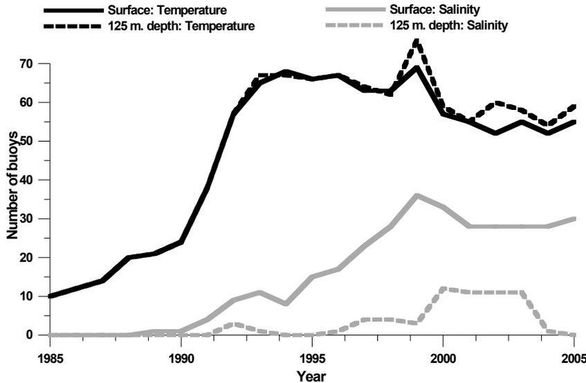
**Figure 8** Number of TAO/TRITON buoys with temperature and salinity (conductivity) sensors by year. The present total number of buoys reporting ocean temperature or salinity is 68. The count for 1999 is > 68 due to switch from TAO to TRITON buoys in the western Pacific.
