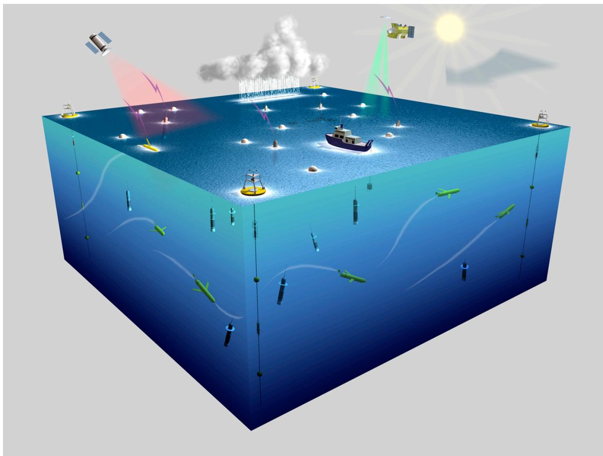
**Figure 12.** Schematic showing floats, drifters, gliders, moorings, ships and satellites sampling a volume of ocean in sufficient density to constrain the upper ocean salinity budget and thus the surface freshwater flux. Gliders patrol the boundaries, floats and drifters monitor the interior and flux buoys and satellites assess air-sea interactions.
