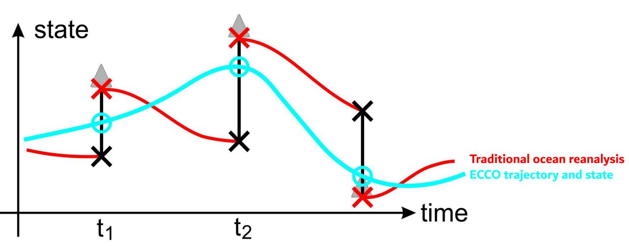
**Inverse problem solved by ECCO:** Solve for a set of *model initial conditions, atmospheric boundary conditions,* and *ocean mixing parameters* such that residuals between the **model solution** and the **observations** are minimized in a least-squares sense.
