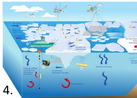
FIGURE 4 | Schematic of the platforms required to observe key sea-ice processes (not capturing circumpolar sea-ice variability (section 'Toward a Better Understanding of Processes Controlling Antarctic Sea-Ice Variability and Change') and deriving sea-ice thickness and volume (section 'Observing Sea-Ice and Volume')). Due to the remoteness, weather, and hostile conditions of the sea-ice zone, autonomous platforms will be crucial. They include high-wind sensors such as drifting buoys (a), ice-deformation arrays (b), mass-balance and snow-buoy (c), wave buoys (d), and autonomous underwater (e) and (f) and vehicles (g). Observations of snow depth, ice thickness, ice concentration, salt and properties from satellite altimetry, and radars and submersibles (h) are essential for long-term time series. Manned observation platforms include vessels (i) for underway and in situ sea-ice landings (including ROV and deep-sea aircraft (e.g., EMARC and NASA's Operation IceBridge)) and near-coastal research stations for fast-ice and sea-ice/shelf studies. Modified from Minnett et al. (2019).
