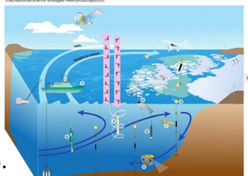
FIGURE 6 | Components of an optimal observing system to constrain and quantify biogeochemical cycling processes in the Southern Ocean. New methodologies such as biogeochemical sensors deployed on SOCCOM (a) and SOCOM (b) floats, gliders (c), and moorings (d), and sampling from ROVs (e) must be integrated with traditional ship- (f) and station-based approaches. Ice-capable tow-Argo floats (g) and biogeochemical sensors deployed on marine mammals (h) are needed to extend the observational range in time and space. Airborne deployment of ALAMO floats (i) could increase spatial coverage substantially. All of these in situ approaches should be combined with existing and improved satellite-based measurements (j) of sea surface height, sea ice, sea surface temperature, and ocean color to develop an integrated biogeochemical observing system for the Southern Ocean. Modified from Minnett et al. (2019).
