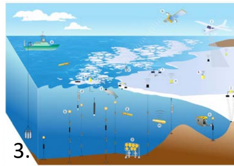
FIGURE 3 | A schematic of the integrated system of observational platforms required to determine the contribution of oceanic heat to ice-shelf melt for a generic configuration. An integrated system to observe the processes important for grounding line retreat and basal melt consists of three main components. First, 'how ocean currents approach and melt the ice shelf cavity, achieved by a combination of ship-based observations, such as hydrographic sections (a), (b), (c) and ice mass buoys (d) particularly in fast- or multi-year ice, sea tags (e), and gliders (f) for high-resolution tracks on the shelf and slope. Secondly, 'gl changes in ice shelf thickness, basal melt rates, and grounding line retreat, achieved by deployment of satellite (g) and airborne (h) remote sensing for ice. APRES radars (i) for direct basal-melt rates, automatic weather stations (j), GPS, barometers, and other sensors (k) for other properties, such as snow accumulation. Finally, observation of processes within the ice shelf cavity itself requires AUVs (l) for observations of water properties, as well as swath mapping of sea floor and sub-ice shelf topography; sensor/mooring deployed through icebergs (m) for sub-ice shelf properties, circulation, and direct basal melt data, including mooring with ITPs and telemetry; moorings deployed by ROVs in ice shelf cavity (n), which is not currently implemented but is a promising technological advance in the coming decade; and bottom landers (o) out the front of the ice shelf for a multitude of roles, such as communication gateways, imaging, water sampling, etc. This figure was modified from Minnett et al. (2019) and Finnis et al. (2014) 'seeing below the ice' 2014 strategy available at https://www.researchgate.net/publication/261111111 .
