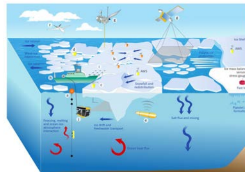
FIGURE 8 | Schematic of the platforms required to observe key sea-ice processes toward capturing circumpolar sea-ice variability (section "Toward a Better Understanding of Processes Controlling Antarctic Sea-Ice Variability and Change") and deriving sea-ice thickness and volume (section "Observing Sea-Ice Thickness and Volume"). Due to the remoteness, vastness, and hostile conditions of the sea-ice zone, autonomous platforms will be crucial. They include high-resolution in situ sensors such as drifting buoys (a), ice-deformation arrays (b), mass-balance and snow-buoys (c), wave buoys (d), and autonomous underwater (e) and airborne vehicles (f). Observations of snow depth, ice thickness, ice concentration, drift and properties from satellite altimeters, and radars and radarsatellites (g) are vital to sustain long-term time series. Maned observation platforms include vessels (h) for underway and in situ sea-ice sampling (i) including ICV (j) (k) (l) (m) (n) (o) (p) (q) (r) (s) (t) (u) (v) (w) (x) (y) (z).
