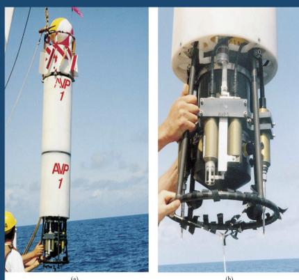
Fig. 2. (a) Absolute Velocity Profiler (AVP) — Autonomous profiler used to measure velocity and density on Blake Outer Ridge. (b) CTD and dual dissipation sensor are shown.
