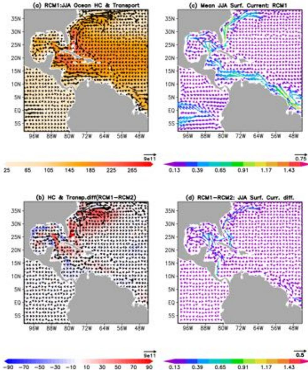
The RCM1 integration (with finer bathymetry) raises the heat content in the IAS and the surface ocean currents are stronger relative to RCM2.
