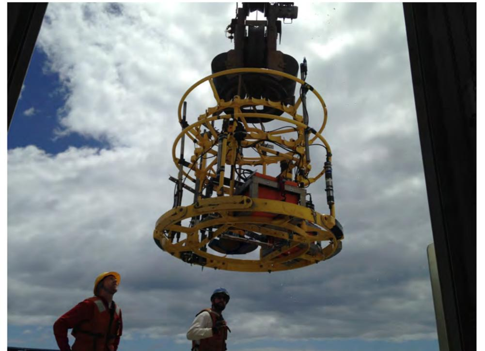
Figure 2: (left) Revelle's deck full of TTIDE mooring gear. (right) The TTIDE CTD with 150-KHz downlooker and Sea Batteries (orange).
