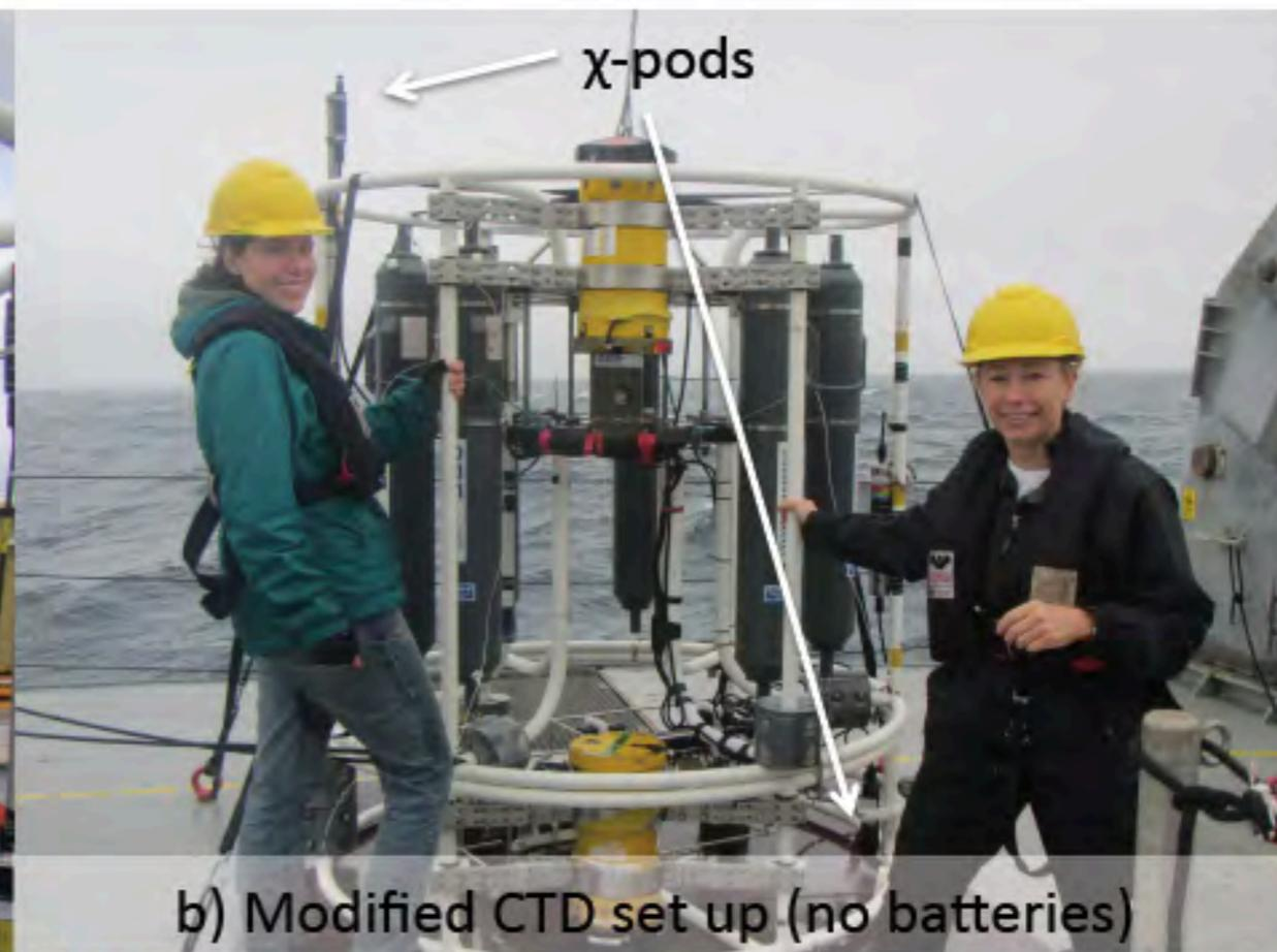
b) Modified CTD set up (no batteries)
