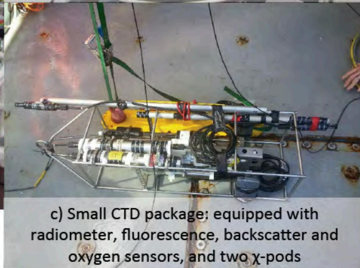
c) Small CTD package: equipped with radiometer, fluorescence, backscatter and oxygen sensors, and two  $\chi$ -pods
