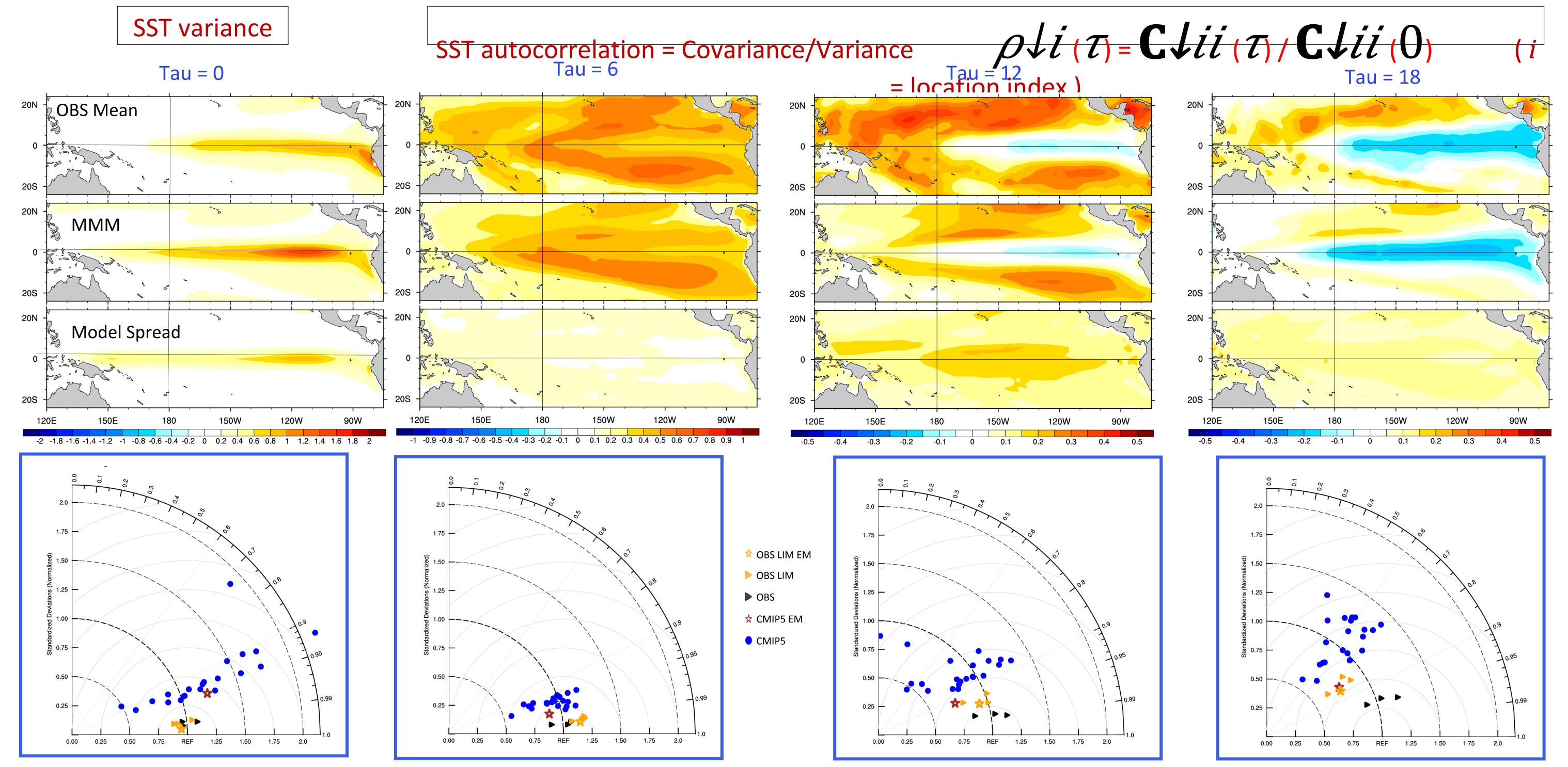
Observational and model monthly SST anomalies have been detrended, and a 3-month running average has been applied prior to the analysis. Taylor diagrams use observational ensemble mean (EM) as reference point and are uncentered (include spatial means).
