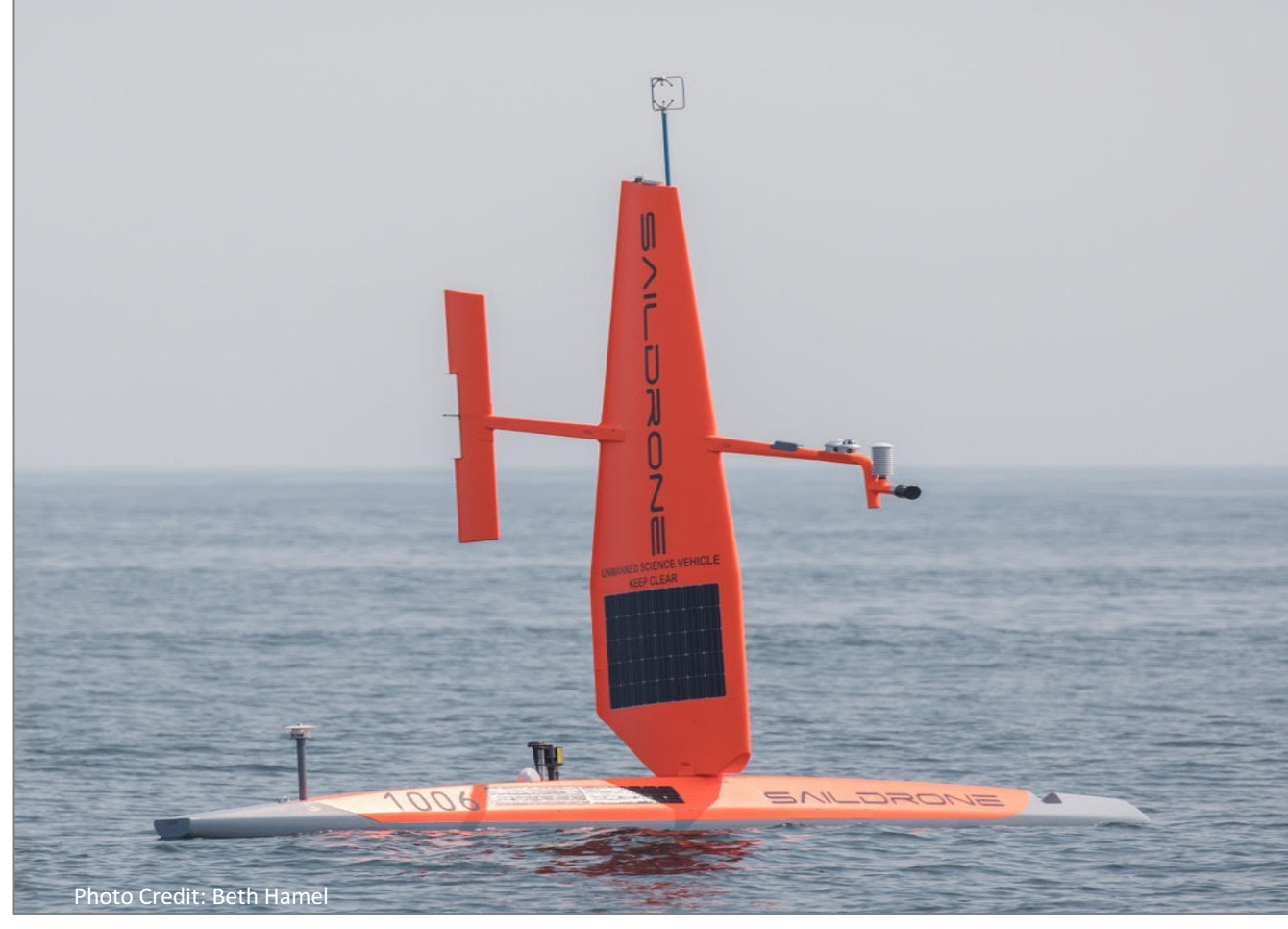
TOP: Third generation Saildrone vehicle. This wing design is too small for effective navigation in the tropics.
