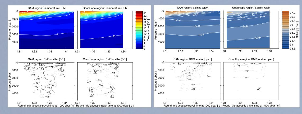
The travel time measurements of the PIES/CPIES can be combined with hydrography-derived look-up tables to estimate full-water-column estimates of temperature, salinity, and density (examples at right). This technique, termed the Gravest Empirical Mode (GEM) method, has been carefully validated through comparison to direct observations on tall moorings at numerous locations around the globe.
