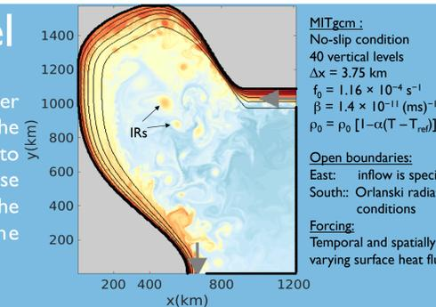
Fig.1: Snapshot of the sea surface temperature (SST) taken after a 15 year spin-up. Black lines denote topography contours with intervals of 500m.
