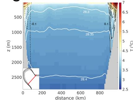
Fig.5: Late spring (May) mean temperature (shading, in  $^{\circ}\text{C}$ ) and density (in  $\text{kg m}^{-3}$ ) over a section indicated by the red line in the inset figure. Positive (negative) velocity contours (c.i. =  $0.1 \text{ cm s}^{-1}$ ) are shown in black solid (dashed) lines.
