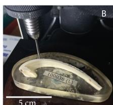
Figure 2. An *A. islandica* shell (A) and a shell cross-section being milled for isotope analysis (B).
