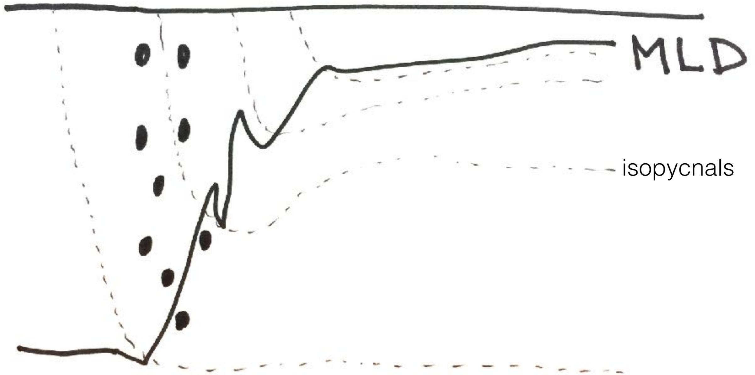
A fleets of low-cost, acoustically tracked Lagrangian floats pre-ballasted to go to a prescribed isopycnal
