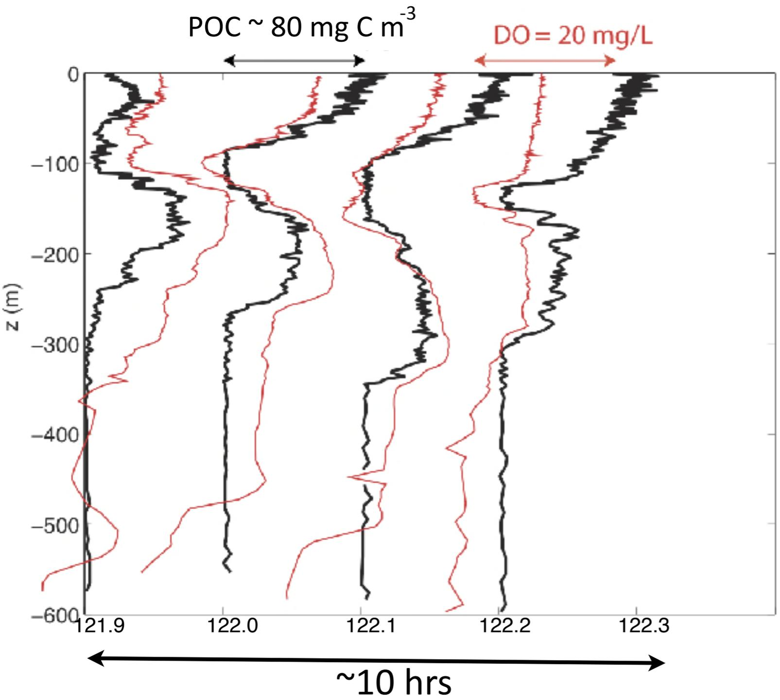
Many Seaglider profiles and CTD casts had subsurface features in optical/BGC properties. ~800 were individually examined for evidence of local, lateral subduction.
