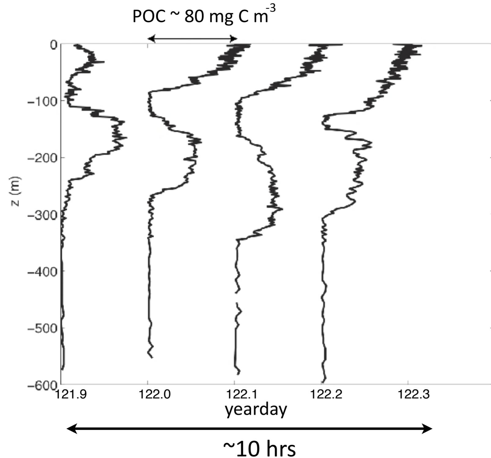
Many Seaglider profiles and CTD casts had subsurface features in optical/BGC properties. ~800 were individually examined for evidence of local, lateral subduction.
