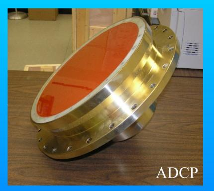
Since 2008 Charlie Flagg and I have been operating an ADCP on the Norröna, a high-seas ferry that operates weekly from the Faroes to Denmark and Iceland. This route spans almost all water flowing towards the Nordic Seas. We give here improved estimates of volume, heat and (fresh water) transport. With an XBT launcher we also routinely sample thermal structure along both sections.
