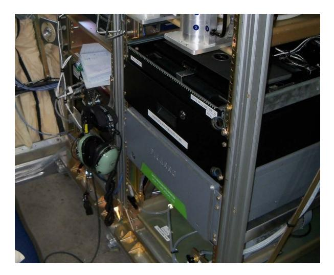
NCAR maintains two flight-ready Picarro water vapor isotopic analyzers for community request. These analyzers pull 0.5 L/min and sample with
