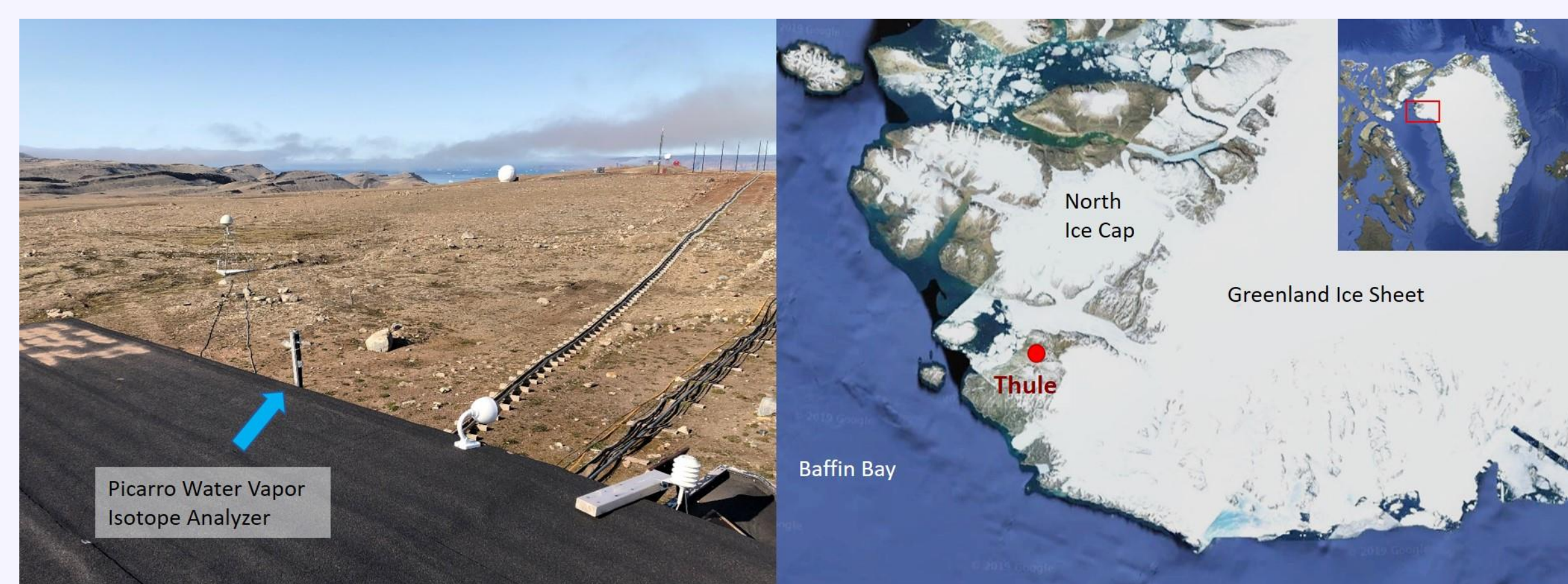
Figure 2. Picarro L2130-i measurement location on roof of 1971 building on South Mountain near Thule Air Base.
