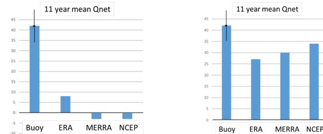
Eleven-year average net heat flux from the NTAS buoy compared to (left) the native fluxes from the models and (right) fluxes computed using the COARE algorithm and surface meteorological variables from the models. Error bars of +/- 8 W/m<sup>2</sup> are shown for the buoy flux.
