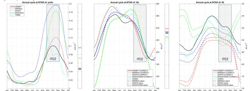
Eleven-year mean annual cycle of (left) precipitation, (middle) shortwave radiation, (right) longwave radiation at the NTAS site from the buoy compared to three reanalysis models. Remote sensing observations from (left) TRMM (middle and right) CERES are also shown. The time period influenced by the ITCZ is shaded.
