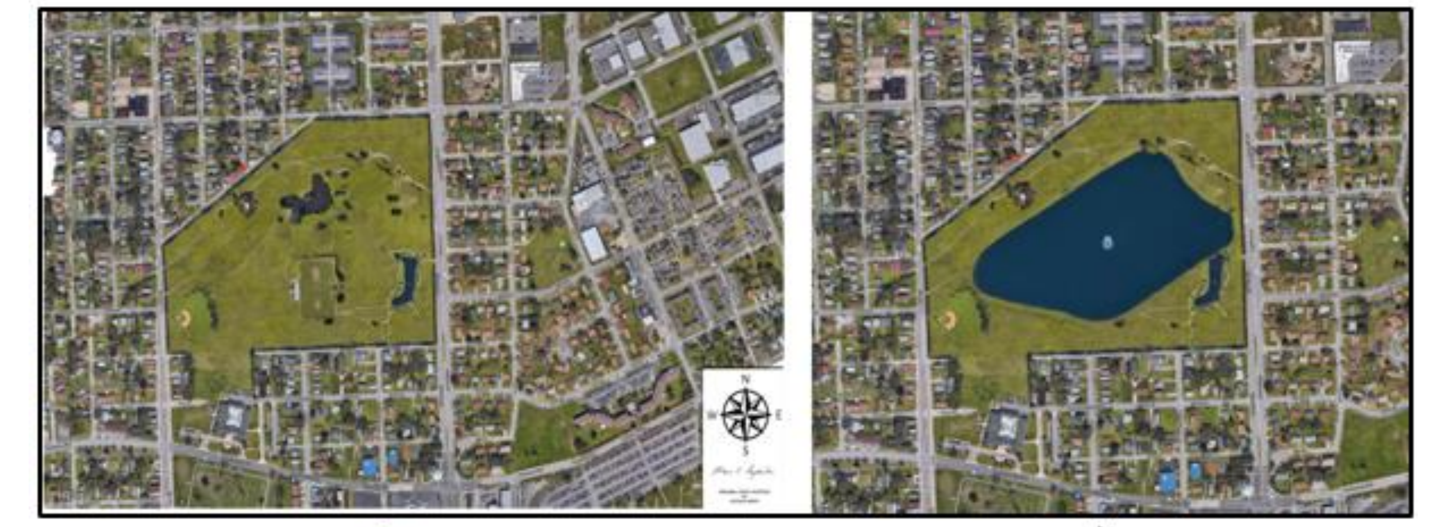
Figure 10: Greenspace with Co-benefit of Recreation (a) and Storm Water Retention (b)
