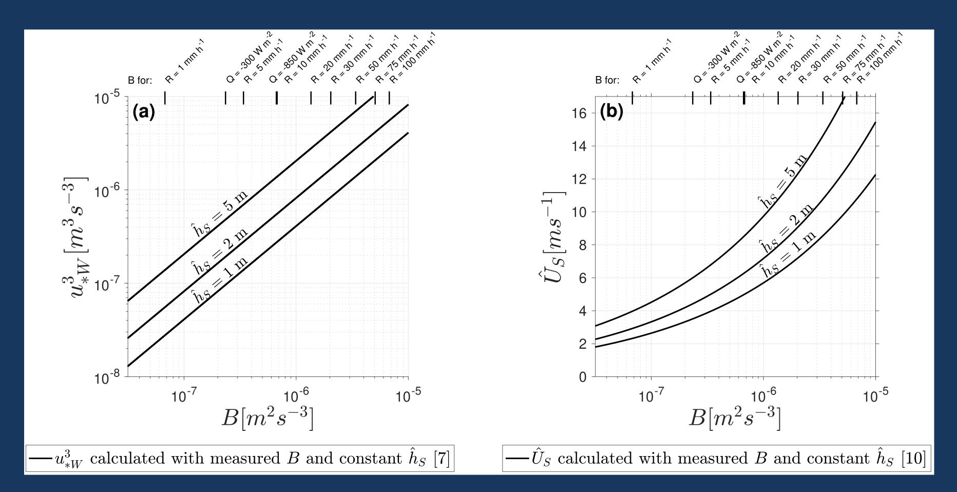
Calculated (a)  $u_{*W}^3$  and (b)  $\widehat{U_S}$  using different stable layer depths of  $h_S = 1$ , 2, and 5 m and measured B. The value of  $\widehat{U_S}$  is the highest value of  $U_{10}$  at which wind mixing and B should support the existence of a stable layer at depth  $h_S$ . Examples of B for various net heat fluxes ( $Q_{\rm Net}$  abbreviated as Q in plot) and rain rates (R) are shown for reference.
