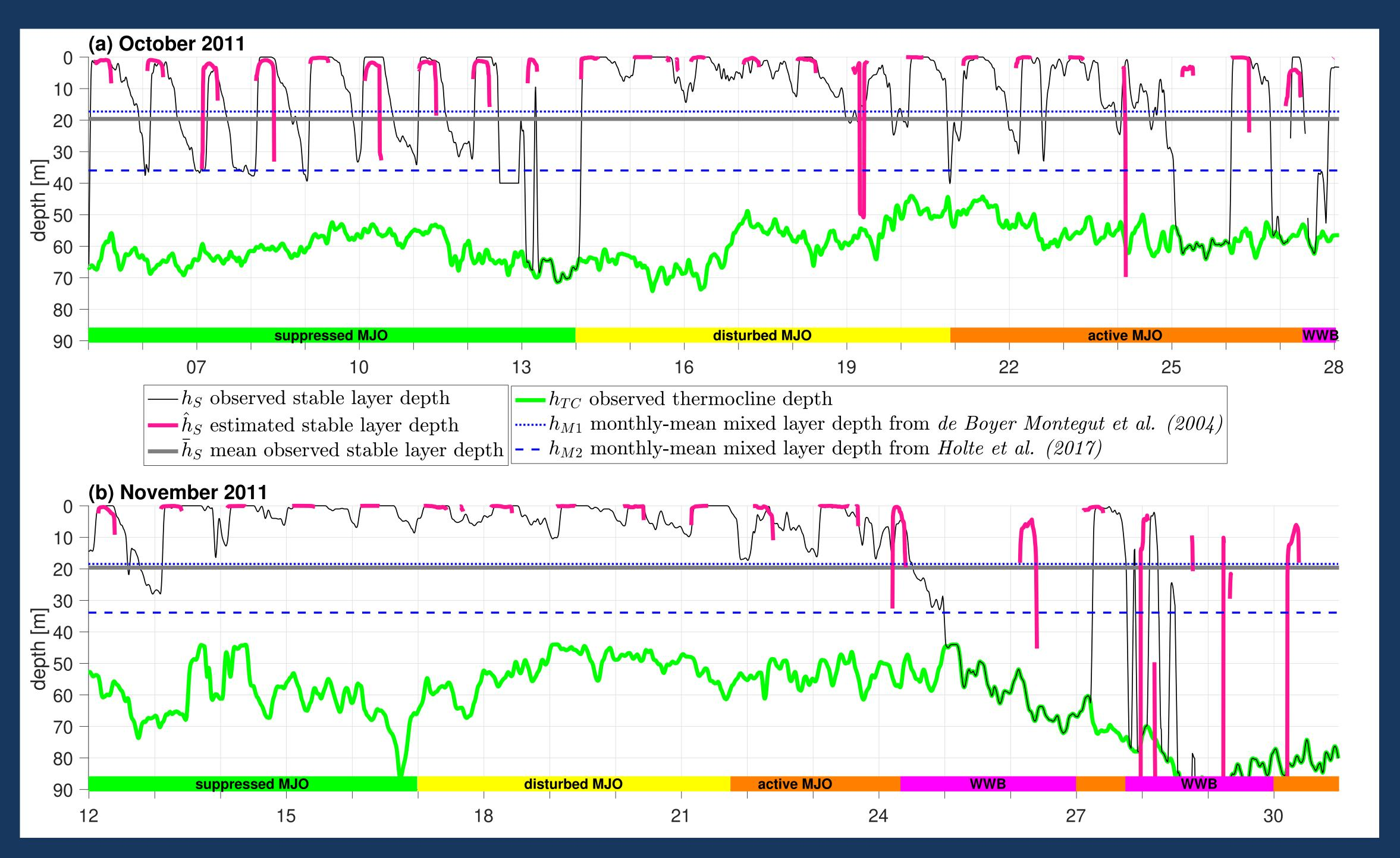
The shallowest stable layer depth in the ocean was determined and tracked from DYNAMO in situ T and S observations from Chameleon profiler. From the 10-m adjusted wind speed,  $U_{10}$ , and surface buoyancy flux, B, we derived estimates of  $\widehat{h_S}$ , ocean stable layer depth (pink), and compared these estimates to DYNAMO observations (black, green) and monthly mixed layer climatologies (blue).
