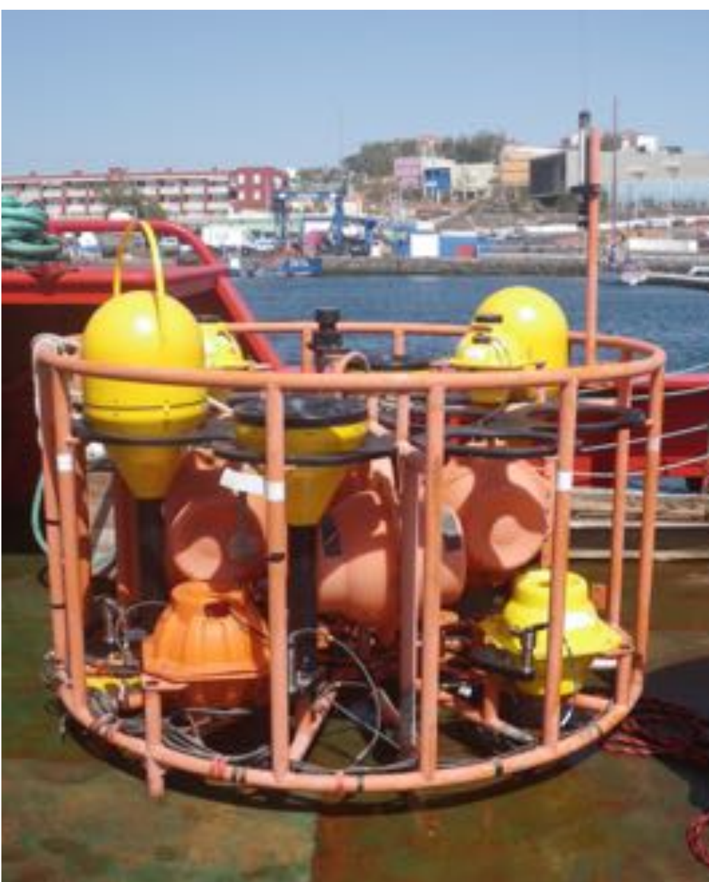
The MYRTLE-X lander after recovery from trials. The electronics are housed in glass spheres at the bottom with some unreleased data pods still attached at the top. Frame buoyancy is provided by 17" glass spheres around the middle.
