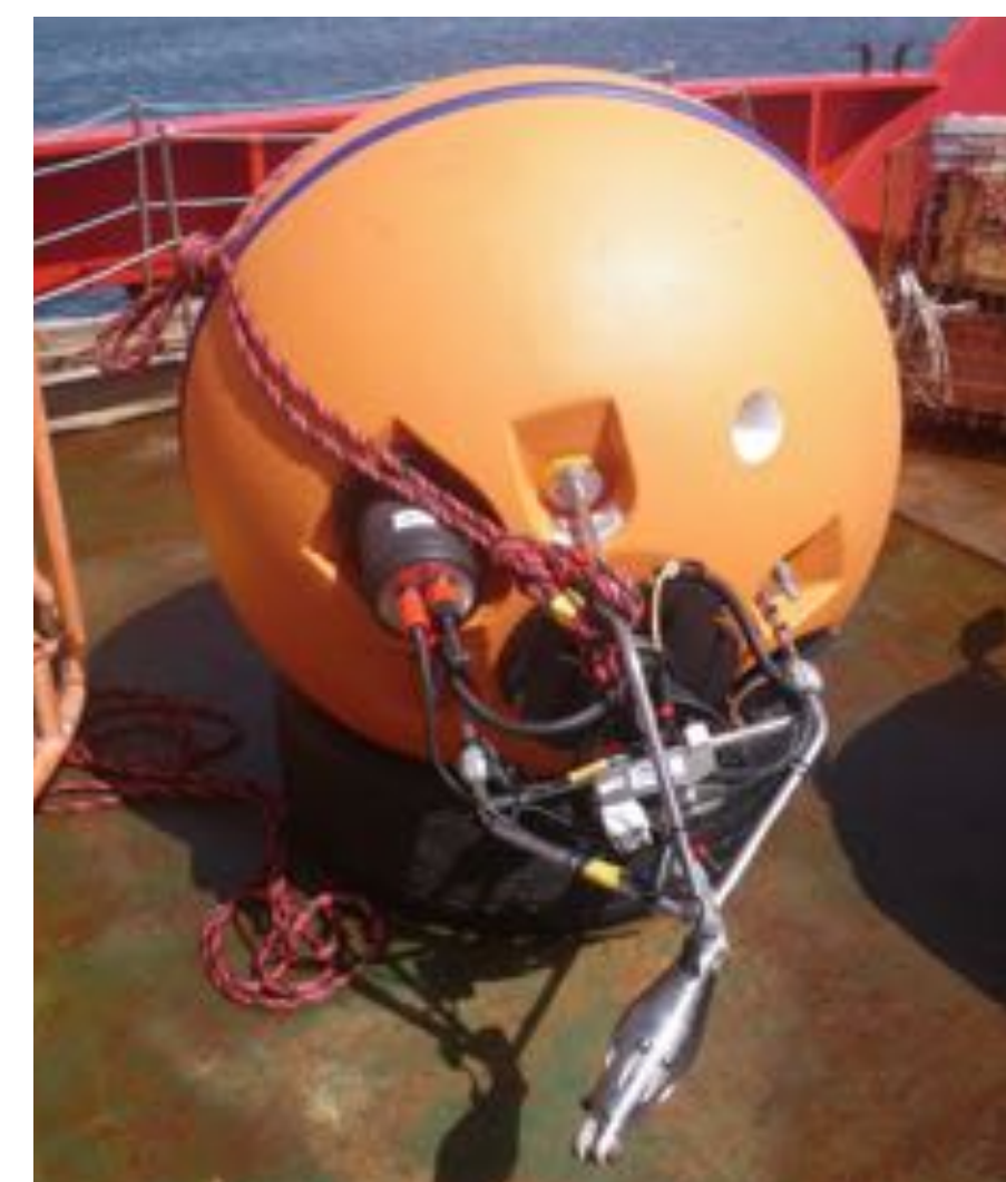
The mooring controller housed in a syntactic float with a Benthos acoustic modem, Inductive Cable Coupler and inductive swivel.
