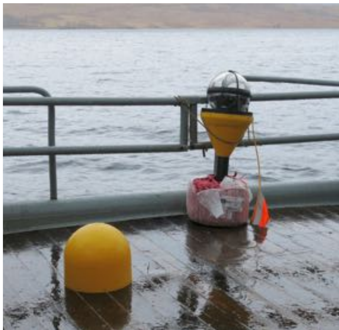
A data pod stood in a coil of rope after recovery during trials. The plastic hard hat has been removed, showing the glass sphere housing the electronics.
