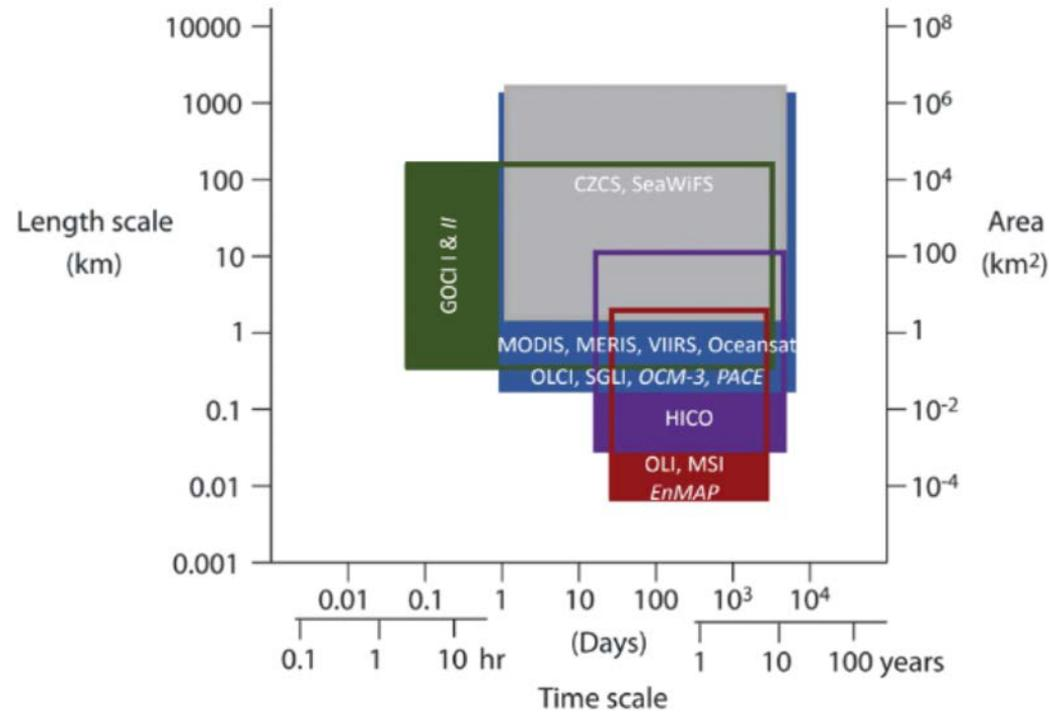
**Figure 2.6** Spatial and temporal resolution of heritage, current and planned ocean colour satellite sensors. Planned sensors and missions are italicized. Note: OLI and MSI are instruments developed for terrestrial observations that have demonstrated success in some coastal applications. Adapted from Mouw et al. (2015).
