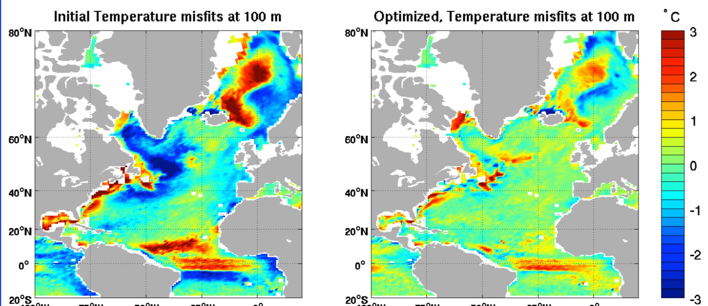
Temperature misfits for (left) "first-guess" solution and (right) optimized ECCO v4 solution at 100 m depth for all in-situ data (Argo, CTDs, XBTs, SeaOs) averaged over 1992-2010. Misfits are calculated as the sample mean for each grid cell of  $T_e - T_o$ , where  $T_o$  are observational profiles and  $T_e$  are the corresponding profiles from the model.
