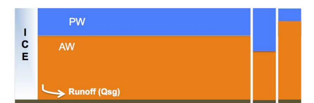
Model geometry and schematic of the periodic boundary conditions at the fjord's mouth with the layer's interface moved upward and downward
