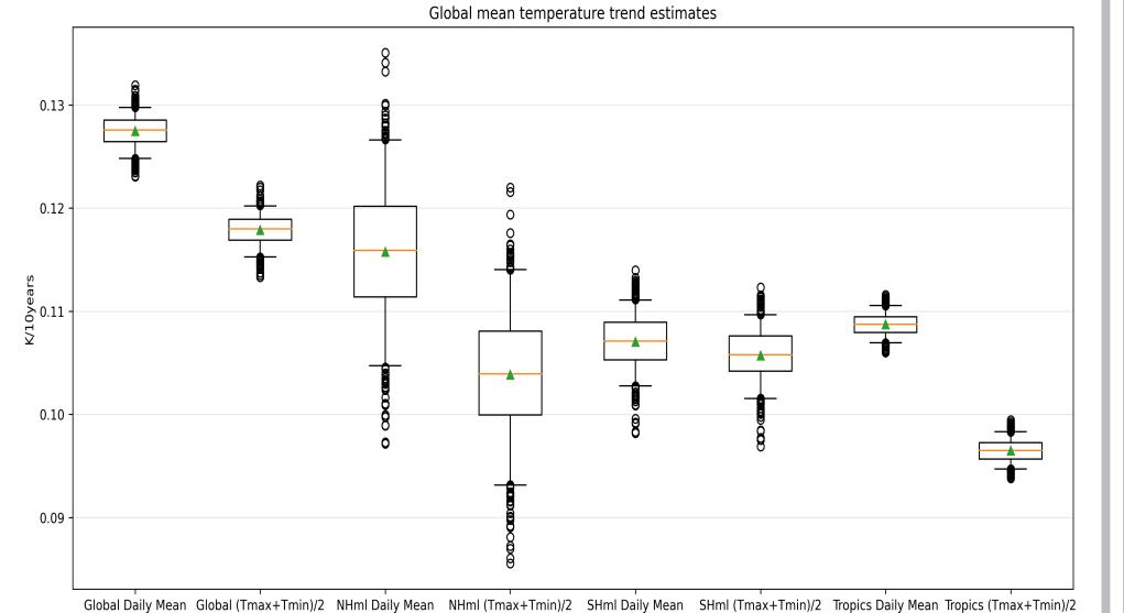
On the global mean scale the trends estimated from  $T_{\text{mean}}$  and  $T_{\text{mm}}$  are significanty different. The difference in global mean temperature trends estimated from  $T_{\text{mean}}$  and  $T_{\text{mm}}$  is about than 0.07K over the 80 years from 1940 - 2019. In South-East Asia this difference comes to 0.8K.
