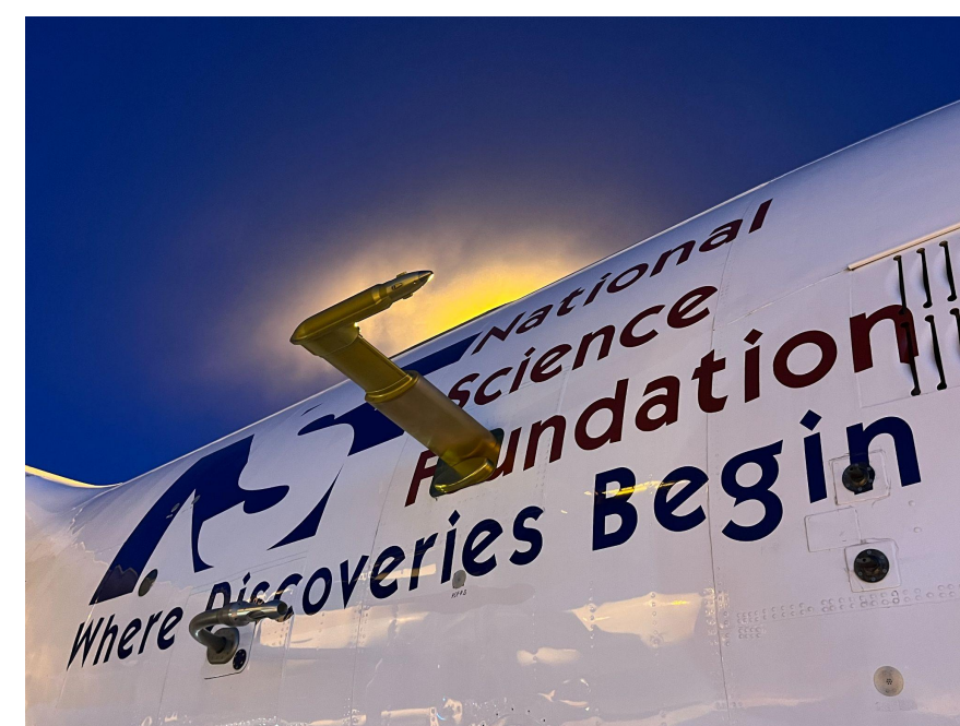
The Counterflow Virtual Impactor (CVI, inlet shown above) separates cloud particles from vapor and aerosol, making it possible to sample isotope ratios in condensate.
