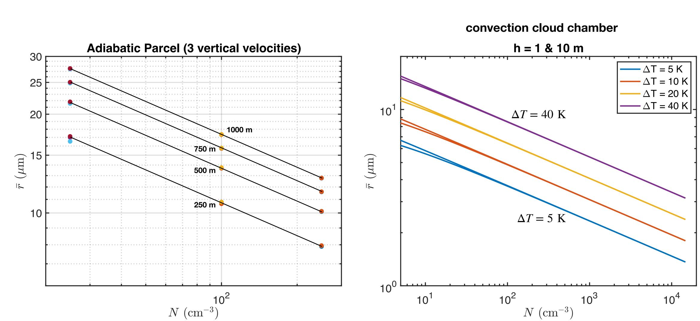
Properties measured at a fixed height above cloud base in an ascending parcel correspond to properties measured at a specific  $\Delta T$  in a convection-cloud chamber.
