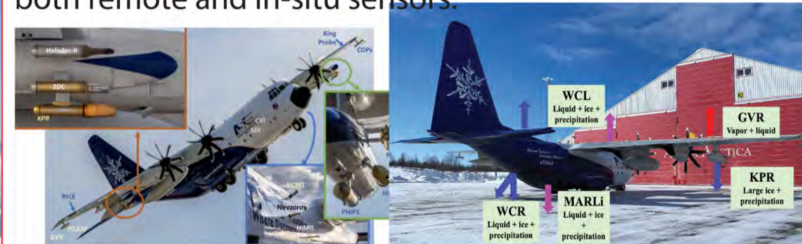
Fig. 2: A strength of CAESAR was its comprehensive suite of instruments. Not shown are the aerosol sensors (CCN, UHSAS, SP2) and trace gas sensors (CO, O3, H2O isotopes). Photo credits: Sarah Woods (left), Zhien Wang (right).
