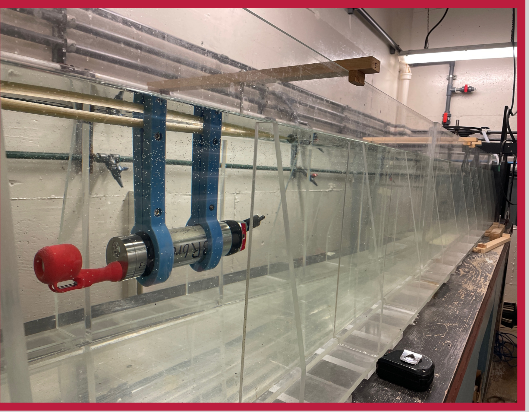
Flume testing to determine thermal inertia coefficients for a range of flow speeds.
