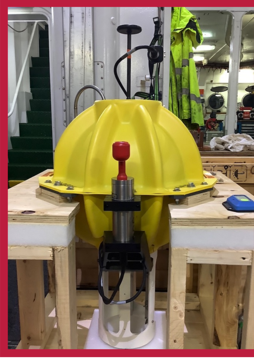
RBRargo 3 |deep6k mounted on a Deep Argo float. Photo Brian King (NOC)
