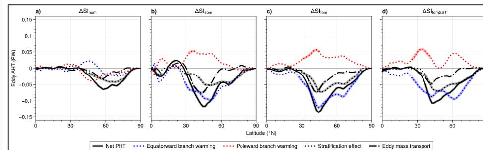
**Figure 4.** Annual mean eddy moist static energy transport. Net eddy AHT response to Arctic sea ice loss (solid black), effective stratification contribution (dotted black), eddy mass transport contribution (dash-dotted black), contribution from the warming of the poleward branch (dotted red) and contribution from the warming of the equatorward branch (dotted blue). (a) Response in NOM. (b)-(d) As in (a) but for SOM, FOM and FOMSST respectively.
