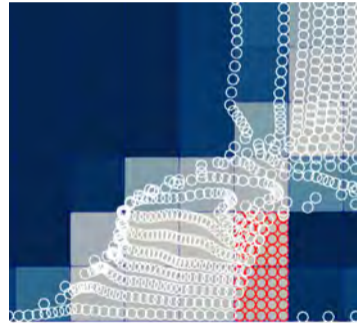
(b) new: with tensile strength for icebergs sea-ice piles up in front of icebergs
