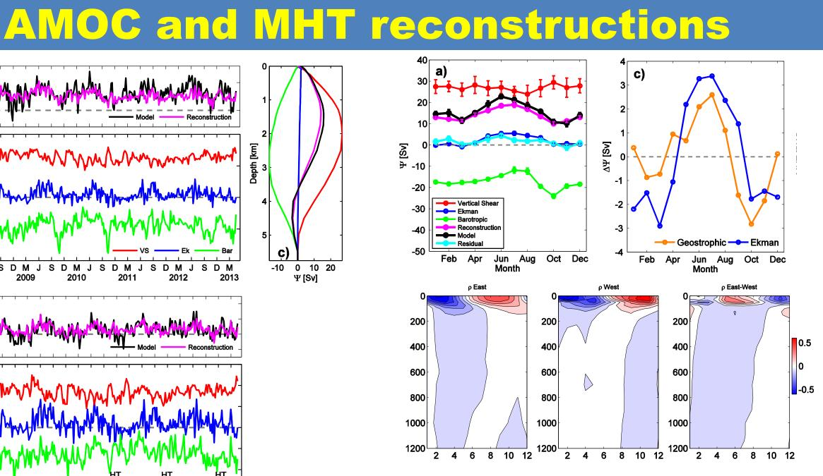
The MOC/MHT reconstructions are decomposed vertical shear, barotropic and Ekman into components. The eddy variability account for most of the residual (reconstruction - model). The seasonal cycle shows Ekman and geostrophic components in phase. Vertical shear has weak seasonal cycle because of strong zonal density compensation.
