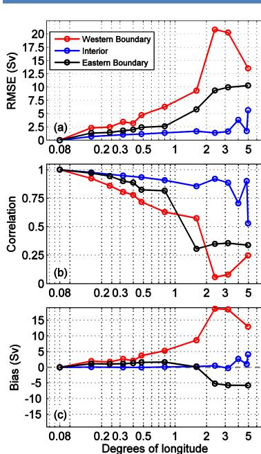
Spatial sampling: The western boundary is the most sensitive to spacing, and the interior the least. Current sampling (25km boundary/50 km interior) is close to optimal.
