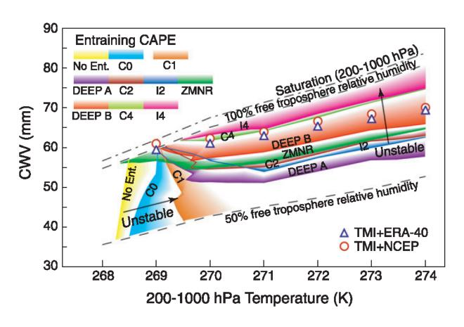
Convective onset column water vapor content as a function of tropospheric temperature and treatment of entrainment
